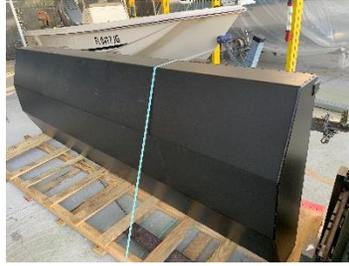
For the new gas tank, Tony decided to have it built using heavier gauge aluminum and coated it for extra corrosion protection.
